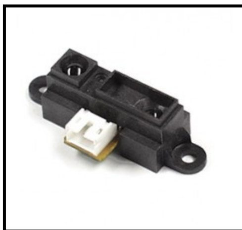
Figure 2.1.1.2 : capteur SHARP GP2Y0A41SK0P
